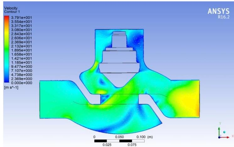
Figure 7: CFD result trial-3 velocity contour
