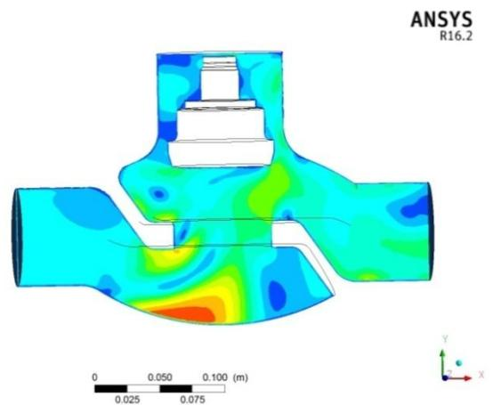
Figure 4: Trial-1 Flat Plug design
