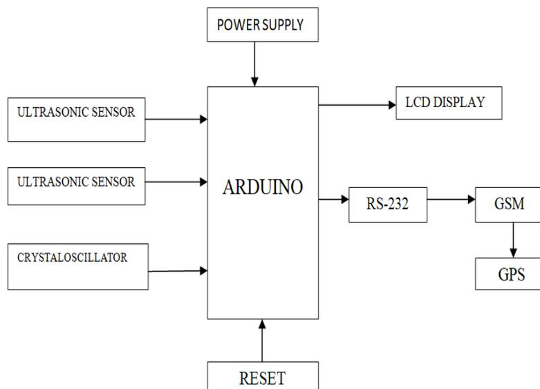
**Figure 1** Block Diagram of proposed system
