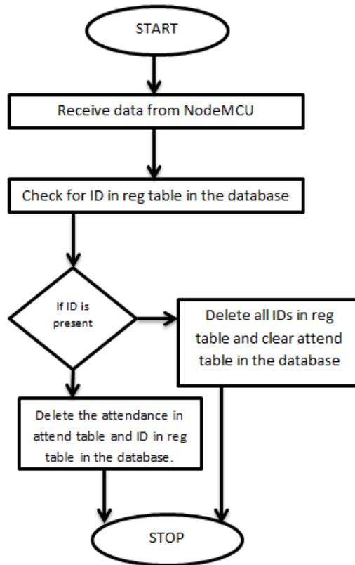
Figure.6 Flowchart of delfinger.php while deleting and reset
