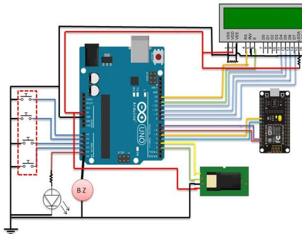
**Figure.1 Circuit Diagram of project**
