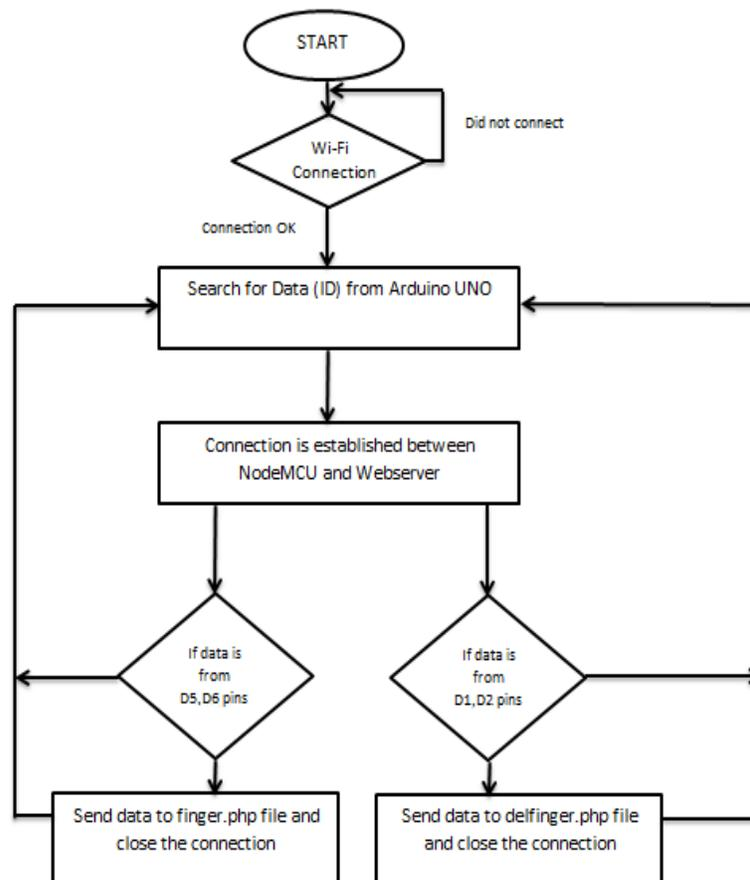
**Figure.4 Flowchart at NodeMCU**
