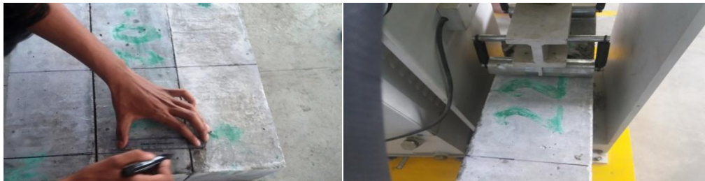
Figure 2 Marking and flexural testing of beams
