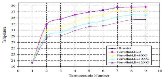
Fig. 2: Magnetic field effect on temperature profile of ferrofluid [4]
