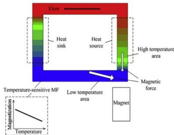
Fig. 4: Working principle of thermomagnetic convection loop[ 6]
