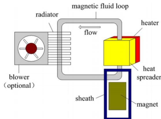
Fig. 3: Schematic layout of the thermomagnetic cooler [6]
