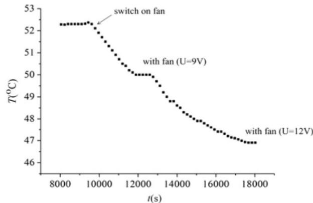
Fig.7 : Temperature drop of the chip surface after the use of fan (2 W heat load) [6]
