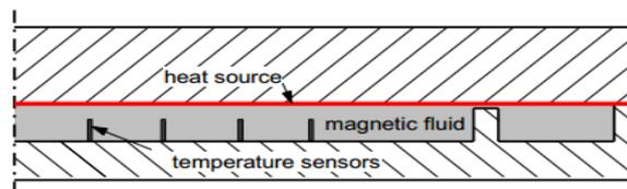
Fig. 9 : Sketch of the measuring cell: measuring volume embedded by two plates
