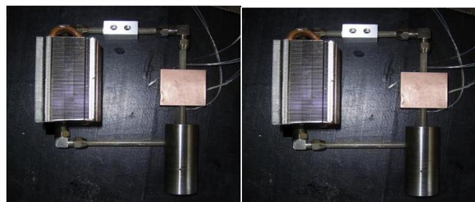
Fig. 5: Prototype of thermomagnetic cooler 1 and2 [ 6]
