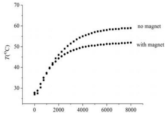
Fig.6 : Averaged surface temperature of the chip (2W heat load)[6]
