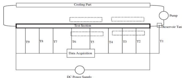
Fig. 1: Schematic representation of experimental set-up [4]
