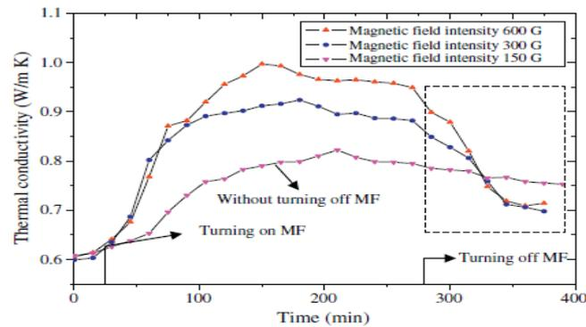
Fig. 8: Thermal Conductivity of ferrofluid versus time under three different magnetic field intensity [7]
