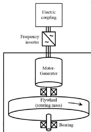
Fig. 1 Diagram of flywheel energy storage system[1]
