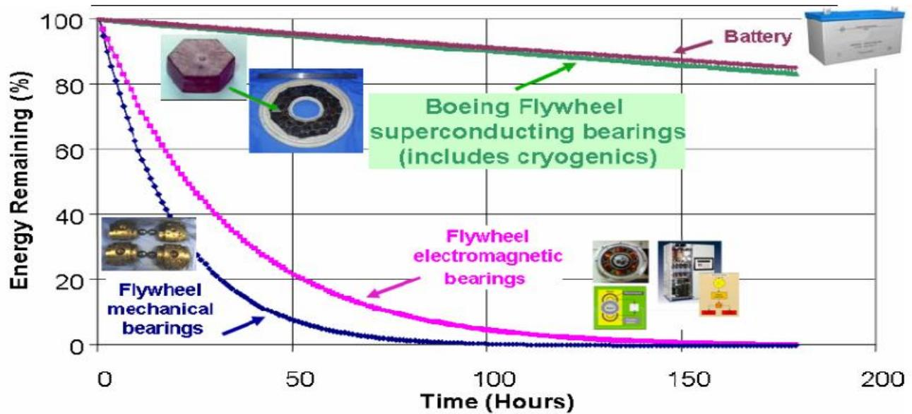
Figure 4: Comparison of FESS with different types of bearings[12]
