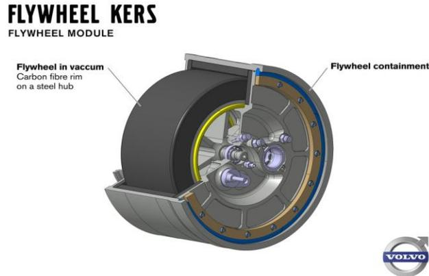
*Figure 7 Volvo's flywheel KERS (APPLICATION IN AUTOMOBILE INDUSTRY)*
