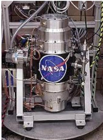
*Figure 6 NASA G2 flywheel for space applications[16]*
