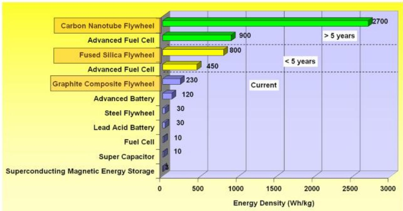
Figure 3 : Comparison of different energy storage systems
