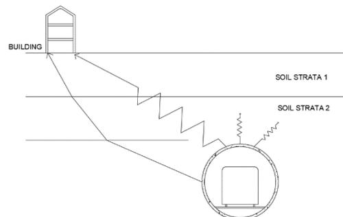
(B) underground metro rail construction vibration
