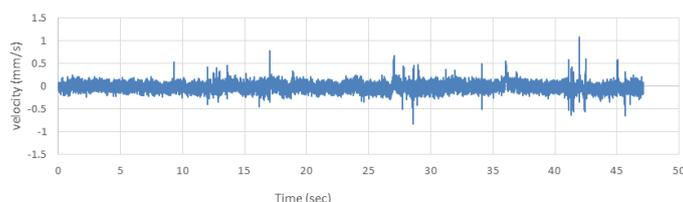
Figure 3 Velocity vs Time for traffic vibration
