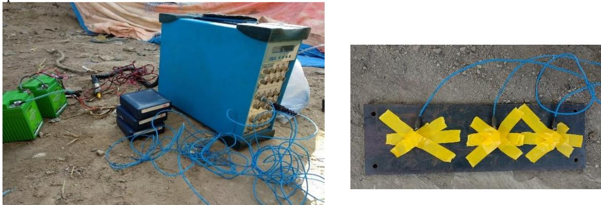
Figure 2 Instrument setup: OROS OR36 analyzer
