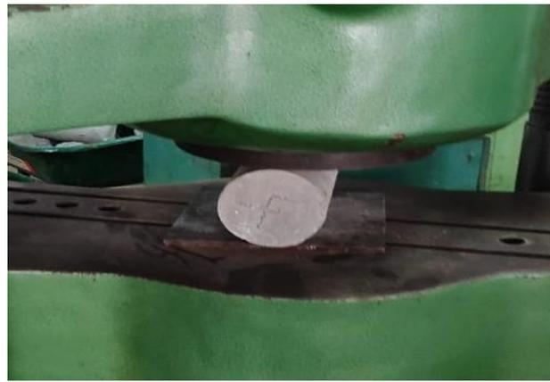
Fig. 5. Optical image of Split tensile strength test
