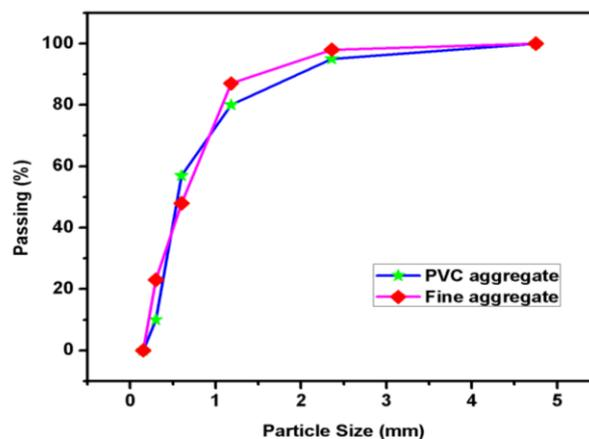
**Fig. 2.** Grading of all types of aggregates
