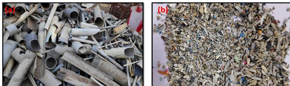
**Fig. 1.** Recycled PVC waste (a) before crushing, (b) after crushing
