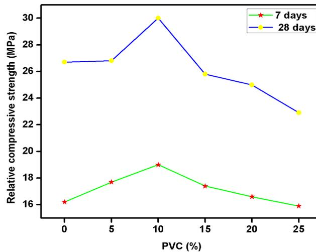
Fig. 4. Relative compressive strength of concrete mixtures
