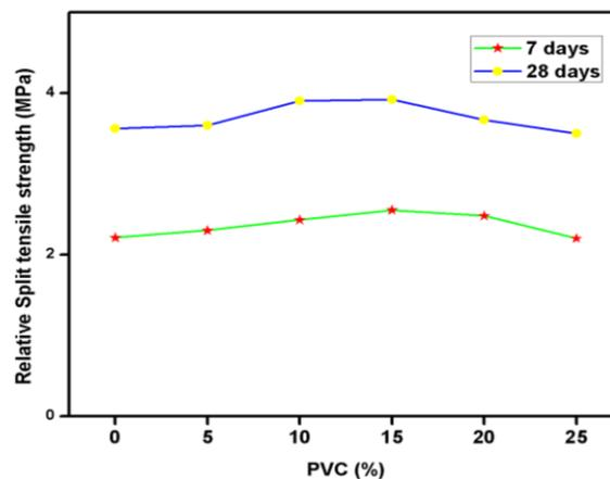
Fig. 6. Relative Split tensile strength of concrete mixtures
