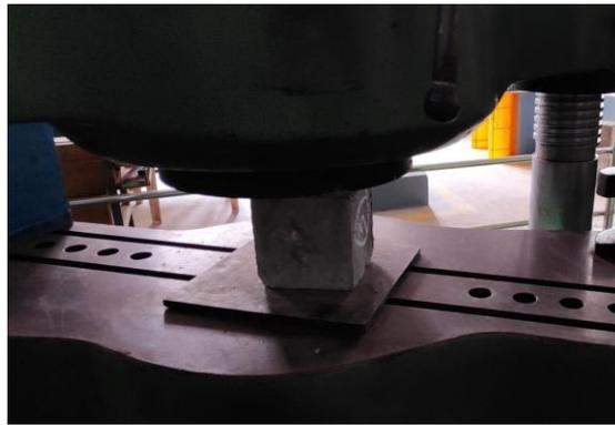
Fig. 4. Optical image of Compression Test
