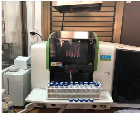
Figure 3 Atomic Absorption Spectrometer
