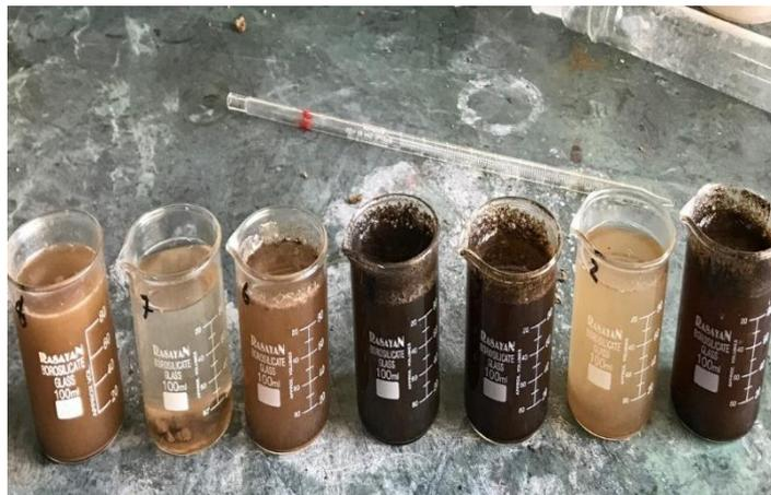
Figure 2 Soil Samples after acid digestion
