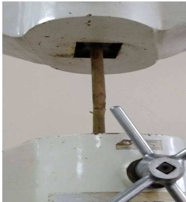
Fig 2 Tension Test Sample 1 While Testing In UTM Machine
