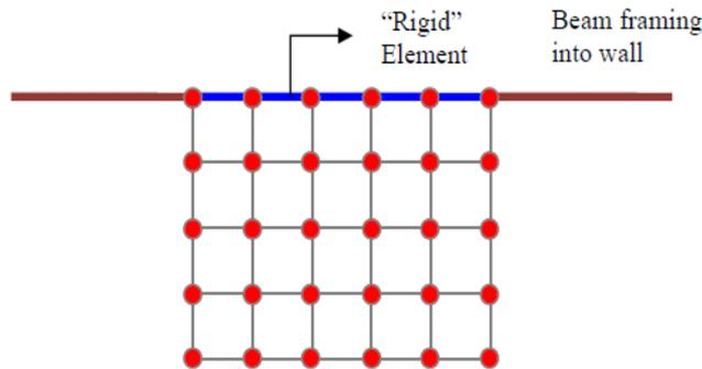
Fig.4-Shell Elements with rigid beams along wall top
