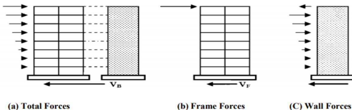
Fig.1 Frame-shear wall structure
