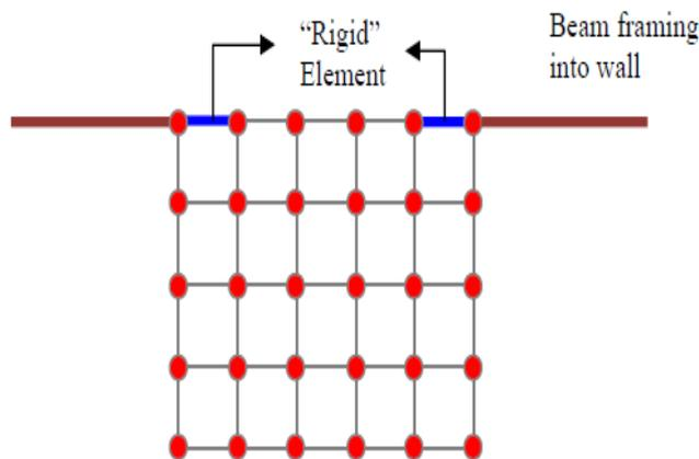
Fig.5-Shell element with rigid beams penetrating along only single mesh
