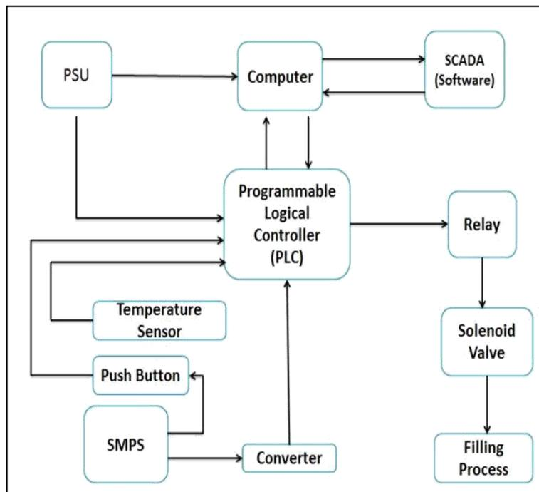
Figure -1: Block diagram
