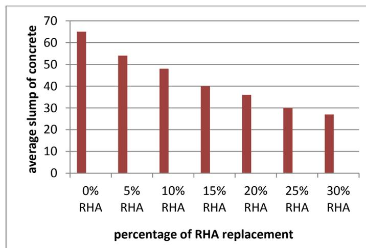
*Fig.1 Workability of Concrete at Different Level of RHA Replacement*
