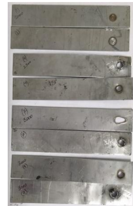
Fig. 5 Medium frequency direct current, Fig. 6 Welded Martensitic SS 410 Coupons Fig. 7 Samples after Tensile Test (RSW) machine
