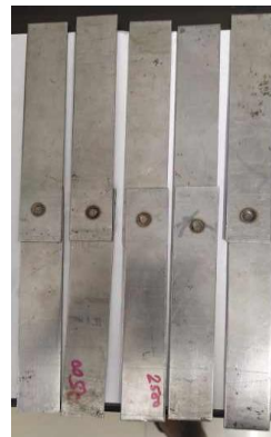
Fig. 5 Medium frequency direct current, Fig. 6 Welded Martensitic SS 410 Coupons Fig. 7 Samples after Tensile Test (RSW) machine
