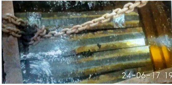
Fig. 11 beams immersed in saline water tank
