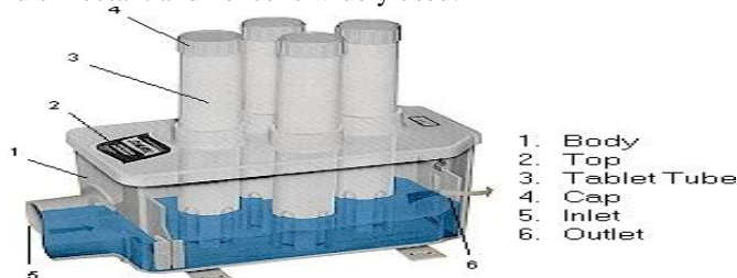
Figure-7- Chlorination unit
