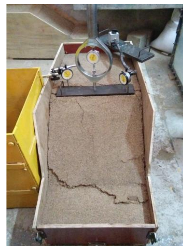
Fig. 7: Slope failed after test
