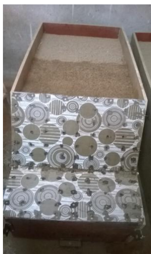
Fig. 5: Injected test slope
