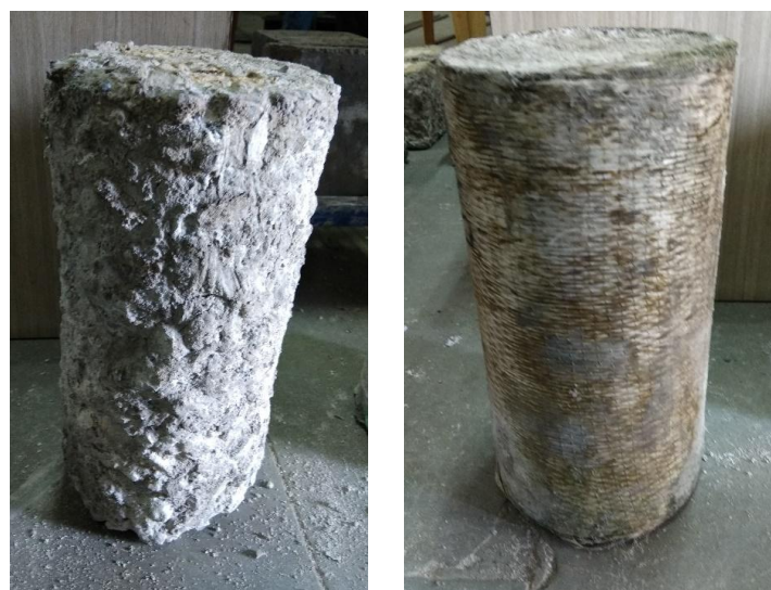
Fig. 5 Acid attack test (a) control specimen (b) GFRP wrapped specimen
