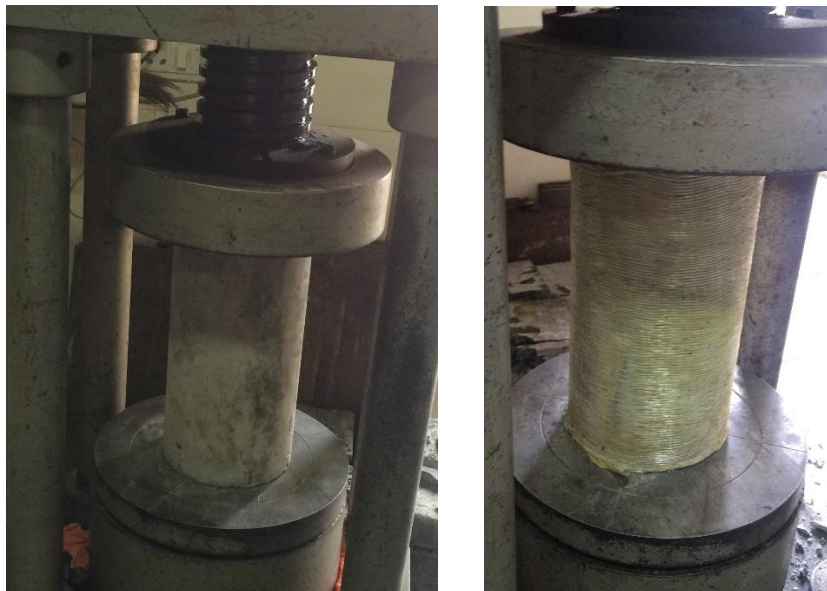
Fig. 1 Compressive strength test (a) control specimen (b) GFRP wrapped specimen
