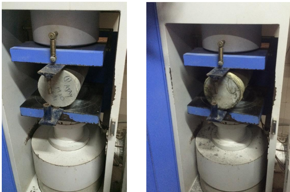
Fig. 3 Split tensile strength test (a) control specimen (b) GFRP wrapped specimen
