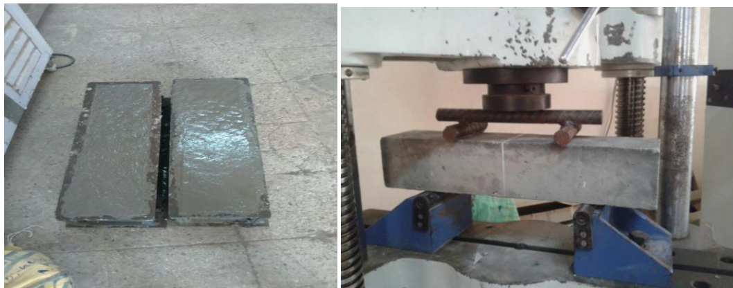
Fig 8.Casting of beams &test in Flexural Strength testing machine
