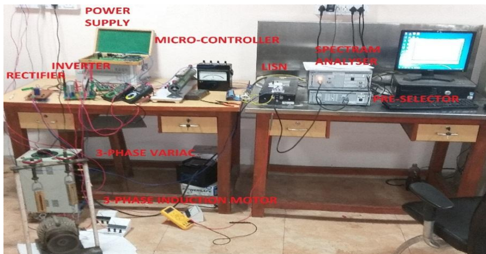
Figure 6 Hardware setup for measuring leakage current and conducted EMI of VFD
