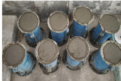
Fig 4: Casting of cylinders
