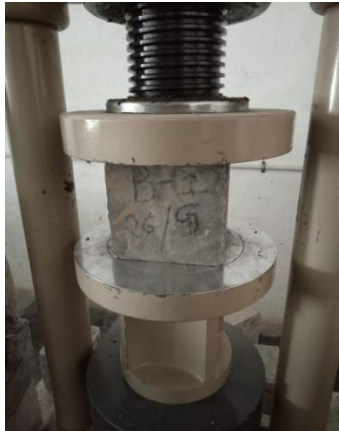
Fig 5: - Compression Test for nGO concrete block
