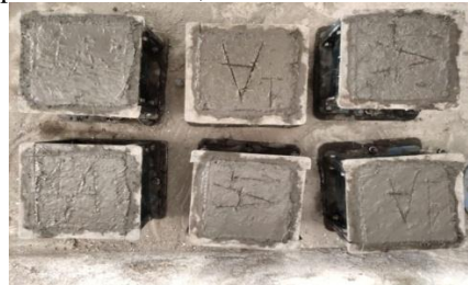
Fig 3: Casting of cubes
