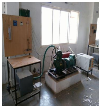
4-stroke diesel engine with electrical loading
