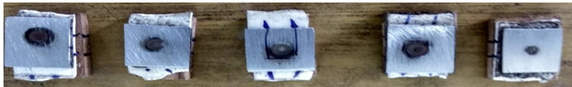
Fig 5 different specimens for corrosion testing
