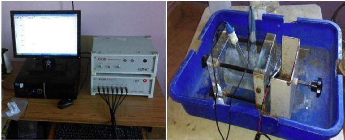
Fig. 5 (a) Equipment for corrosion testing
