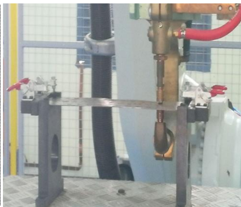
Fig 2 (b) alignment of robot gun to the weld interface
