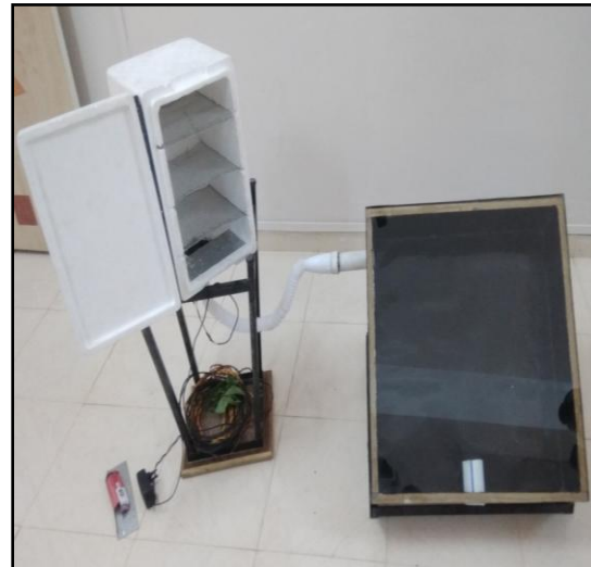
Fig.1.6 Actual View of Mixed-mode Solar Dryer
