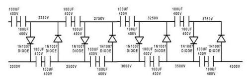
In this circuit diode and capacitor in ladder network. 400v and 100microfarade capacitors are use in this circuit for producing 4 KV. The 1N5400 series is a similarly popular series for higher current applications, up to 3 A. These are fairly low-speed rectifier diodes, being inefficient for square waves of more than 15 kHz.
