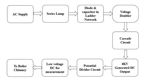
In this block diagram 4kv DC generated from 230v AC supply by using the karl marx circuit. The circuit have a number of diode and capacitors are connected in ladder networks with number of stage. The level of voltage is double in every stage. The output of circuit is very high so it is not possible to measure voltage directly by multimeter. Therefore,
