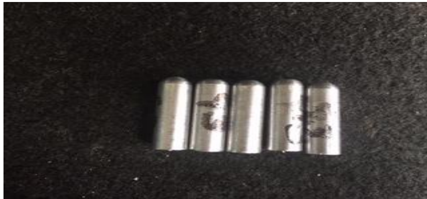
Fig.9. Specimens for wear testing
