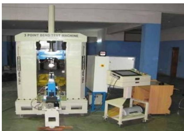
Figure 3: Fracture Test Setup
