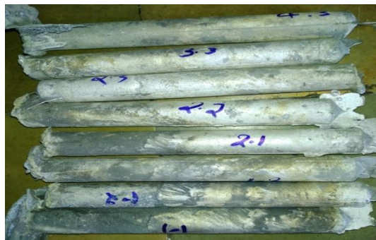
Fig 2.6 Casted cylindrical specimens with different weight percentage of reinforcements
