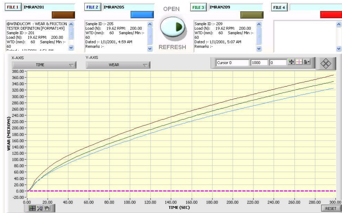
Fig 3.7 Comparison of hybrid composition Mg AZ91D+16% SiC for 1.5% Gr, 2.5% Gr & 3.5% Gr at speed 200rpm.
