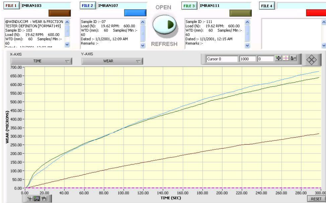
Fig 3.6 Comparison of hybrid composition Mg AZ91D+14% SiC for 1.5% Gr, 2.5% Gr & 3.5% Gr at speed 600rpm.
