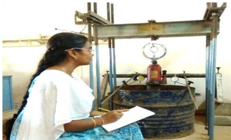
Fig.7 Author conducting cyclic plate load test
