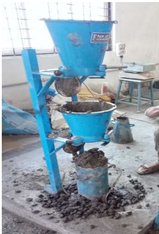
Compaction Factor Test
