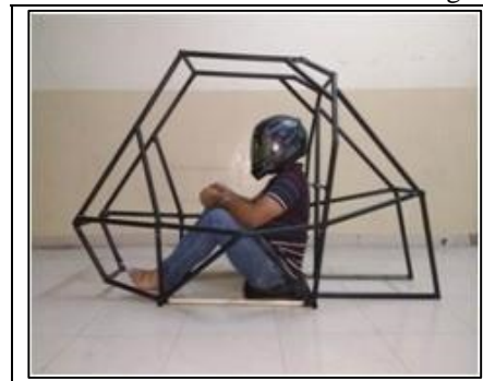
Figure 4: Driver accommodation in rollcage PVC model
