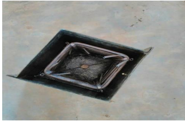
Fig: cube casting for pull out test
