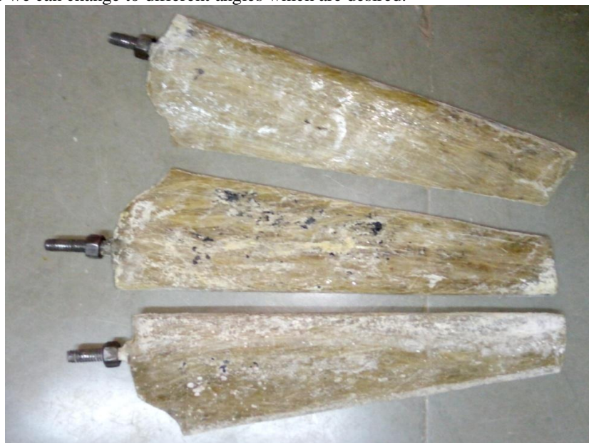
FIGURE.3 Flax fiber with epoxy blades with bolt in bottom
