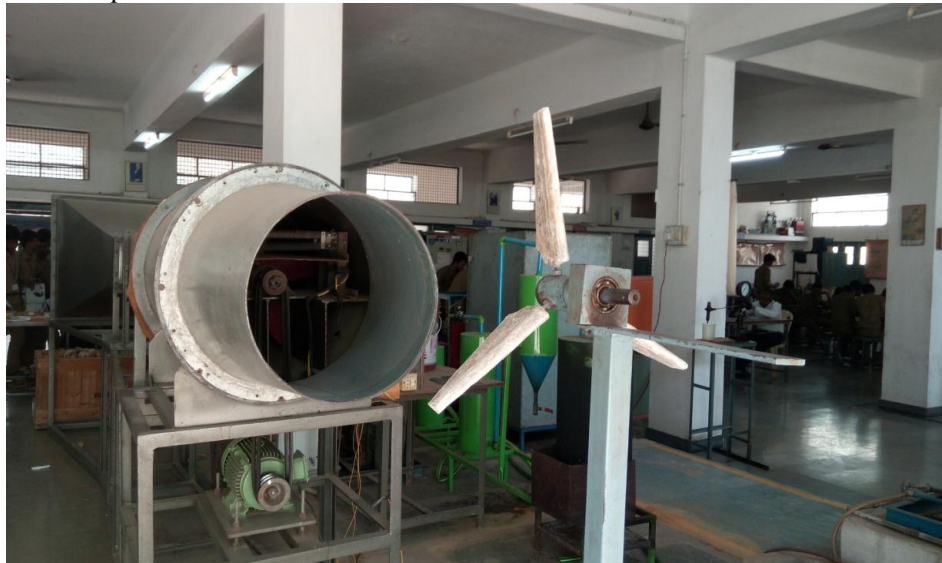
FIGURE.4 wind tunnel with wind turbine made of flax fiber blades
