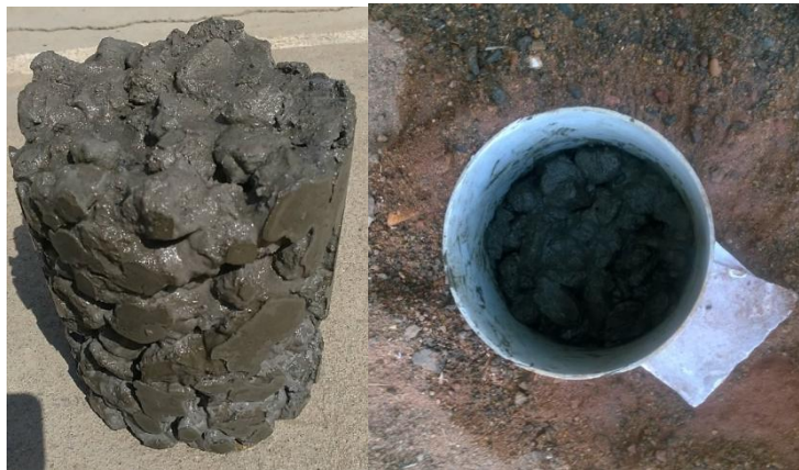
Fig.1 Pervious concrete cylinder Fig.2 Pervious concrete cylinder casted in pipe
