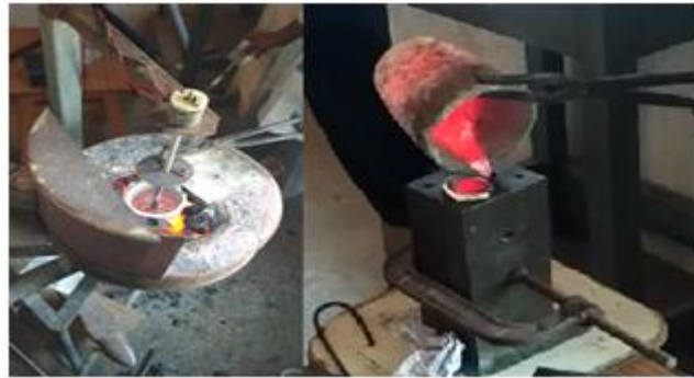
Figure-2: Stir Casting Setup and Casting Mould
