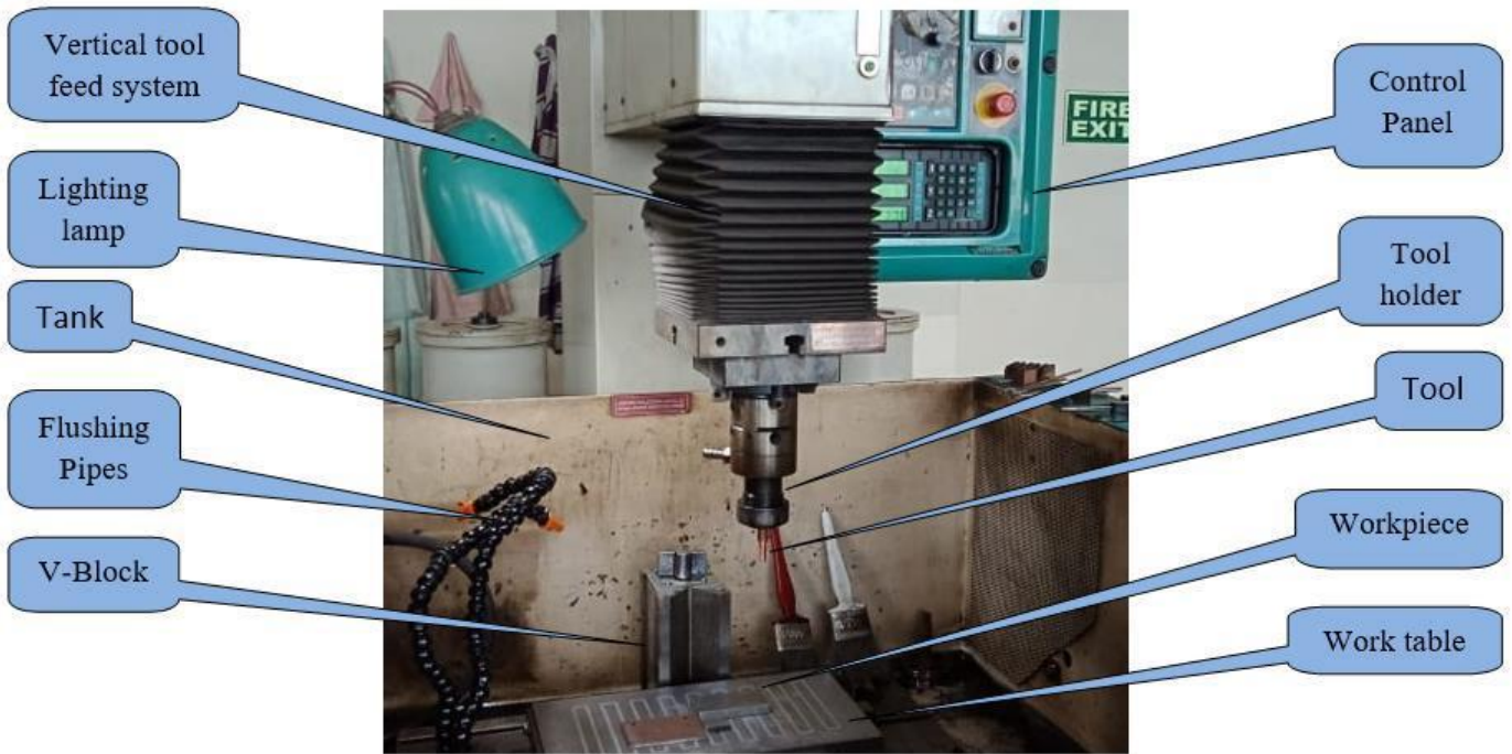
Fig. 2. Schematic diagram of sinking EDM.
