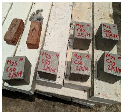
Fig 5: Replacement of Ceramic Sludge into cubes
