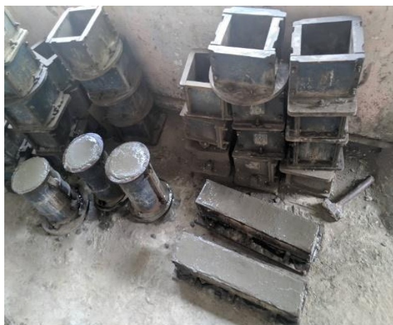
Fig 4: Casting of Beams and Cylinders
