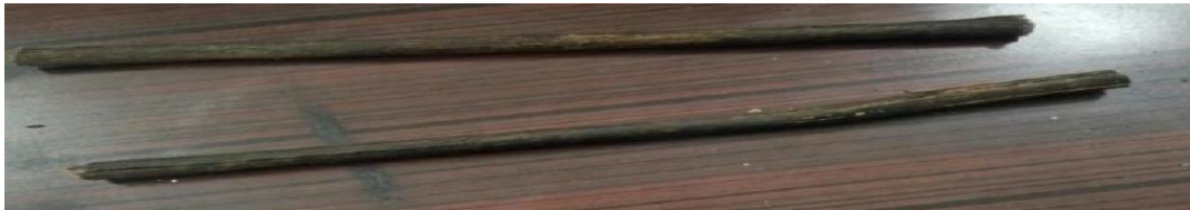
Figure3 : Pultruded jute Carbon fiber hybrid FRP composite rod
