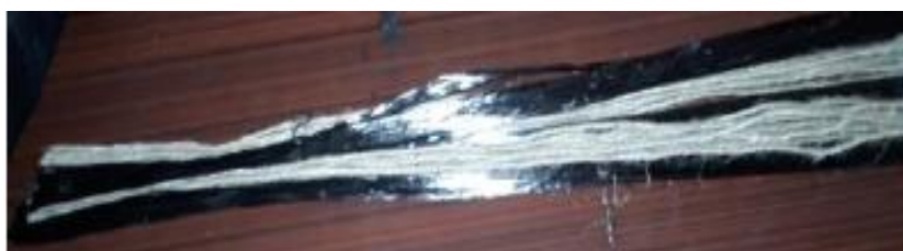
Figure 2: Preformed jute and carbon fiber bundle for pultrusion of hybrid FRP composite
