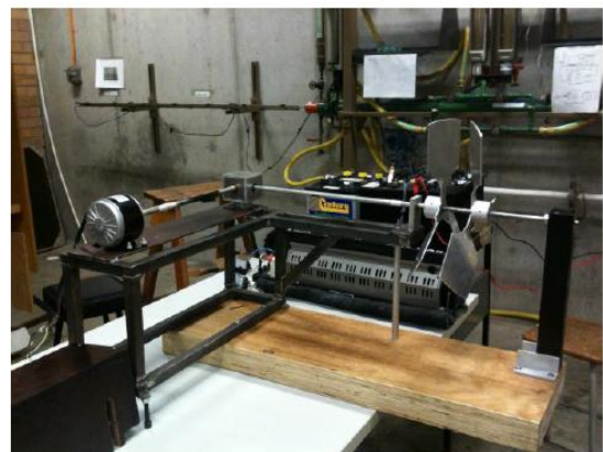
Figure 9. Testing of Coaxial Double Fan (9)
