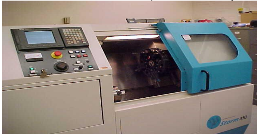
Figure 1: Strom A50 CNC lathe machine with automatic tool changer
