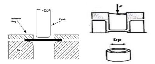
Fig.1 Deep drawing process
