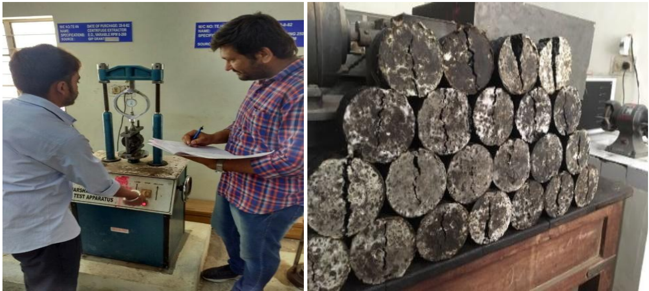
Figure 8 : (a) Indirect Tensile Strength Testing In Progress (b) Failure of Specimens In ITS
