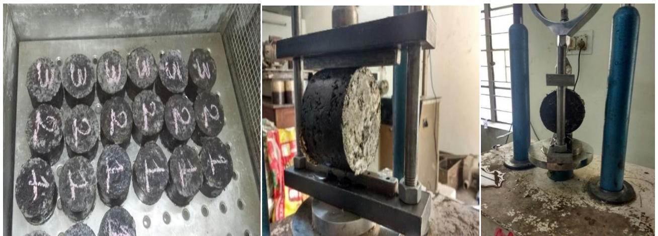
Figure 7 : (a) ITS Specimens In Water Bath (b) ITS Frame (c) Specimen In Frame
