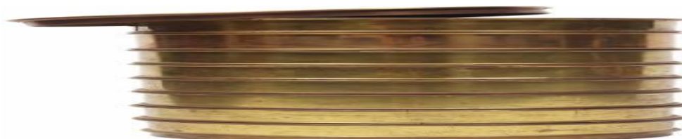
Fig.9 Particle size distribution by sieve analysis:
