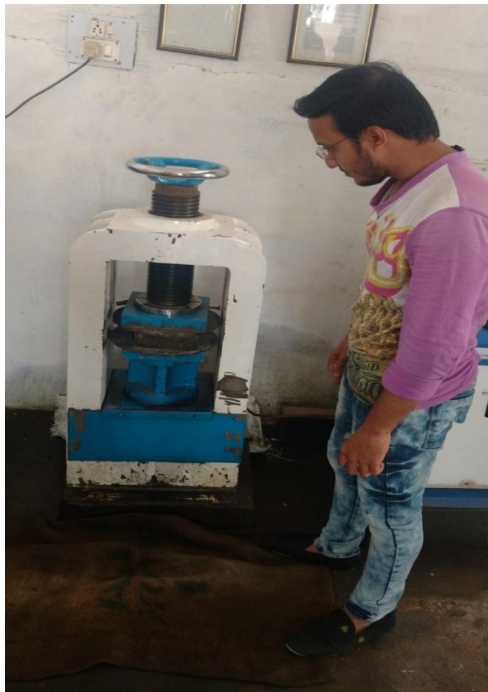
Fig. 3 Compression strength testing of concrete paving block
