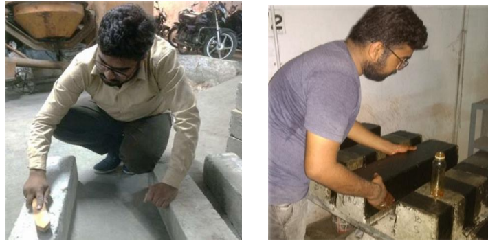
Fig. 5 Surface Preparation and Applying Basalt fiber on Beam.
