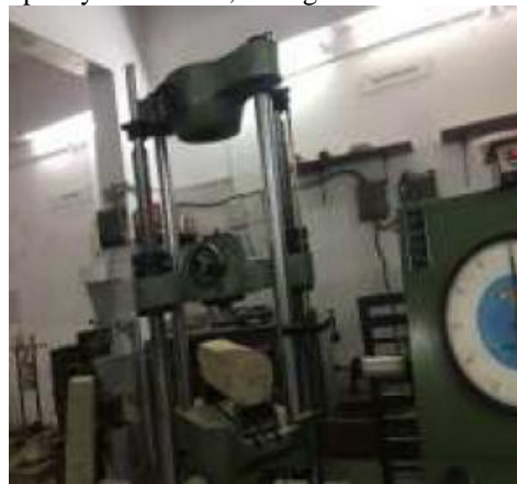
Fig. 3 Beam Testing under (UTM).
