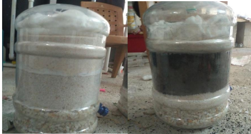
Fig. 3 Arranged Sand and Carbon Filters
