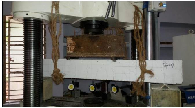
Figure 3 Testing of beam strength
