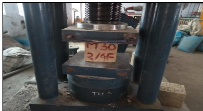
Figure 1 Testing of cube strength
