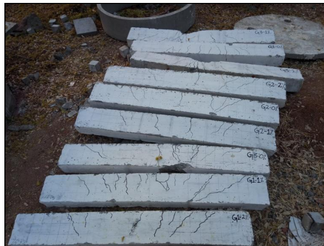
Figure 4 Beams after testing
