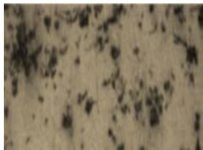
Fig 13: Microstructure of 2 Wt% SiO 2 fortified Al 4032 Fig 14: Microstructure of 3 Wt% SiO 2 fortified Al 4032
