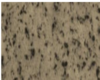
Fig 13: Microstructure of 2 Wt% SiO 2 fortified Al 4032 Fig 14: Microstructure of 3 Wt% SiO 2 fortified Al 4032
