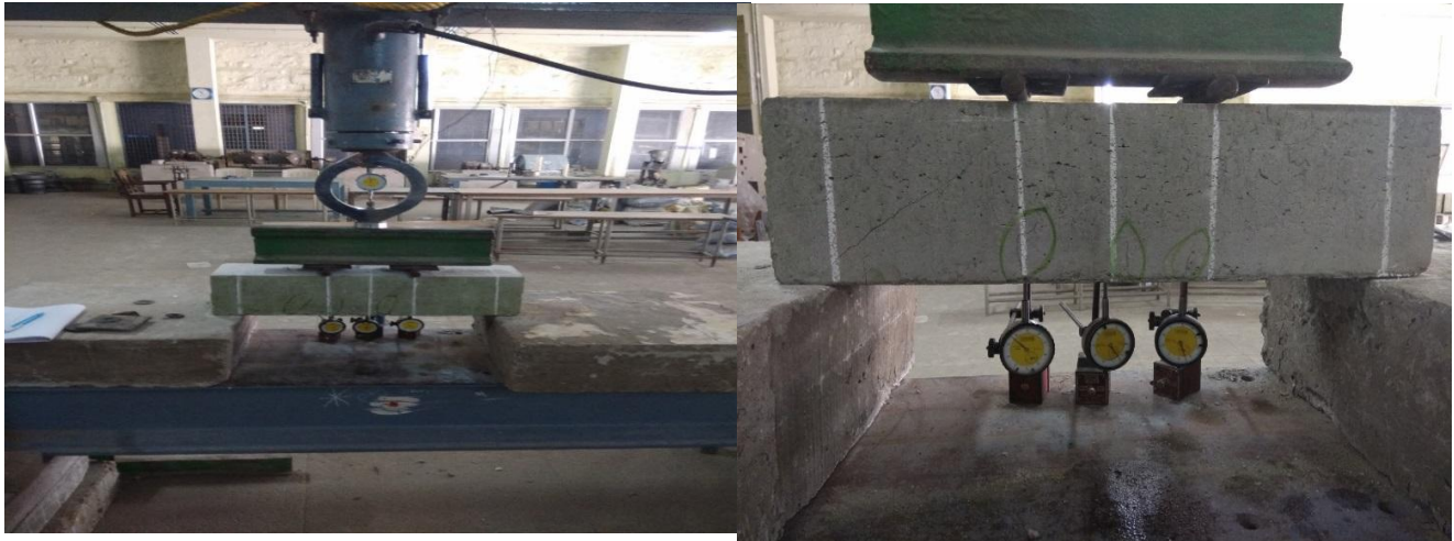
Figure 1: Two point load setup Figure 2: failure of beam under two point load
