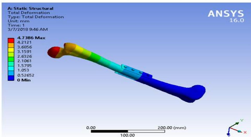
Fig: 4.2.3 picture showing total deformation for model 1 with callus(100%) material
