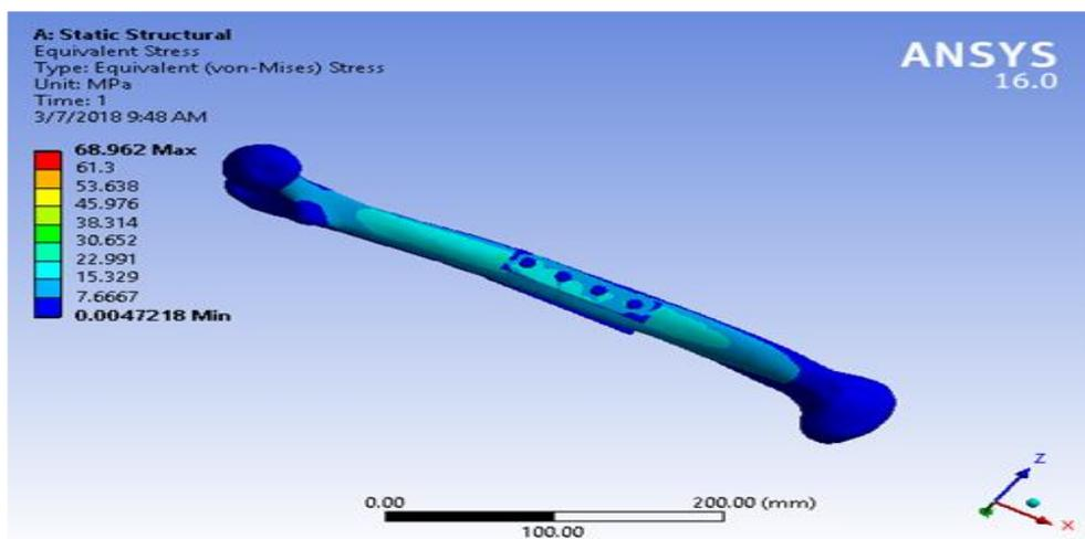
Fig: 4.2.2 picture showing equivalent stress for model 1 with callus(100%)material
