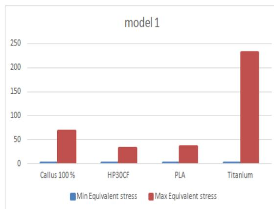
Fig:2 Graph showing Equivalent stress For Model 1 with Different Materials
