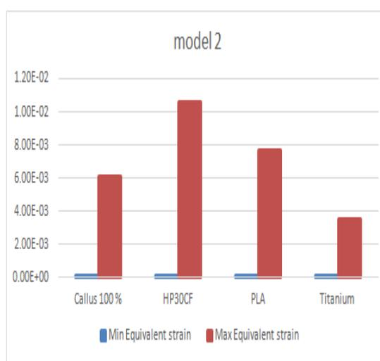
Fig:4 Graph showing Equivalent strain For Model 2 with Different Materials
