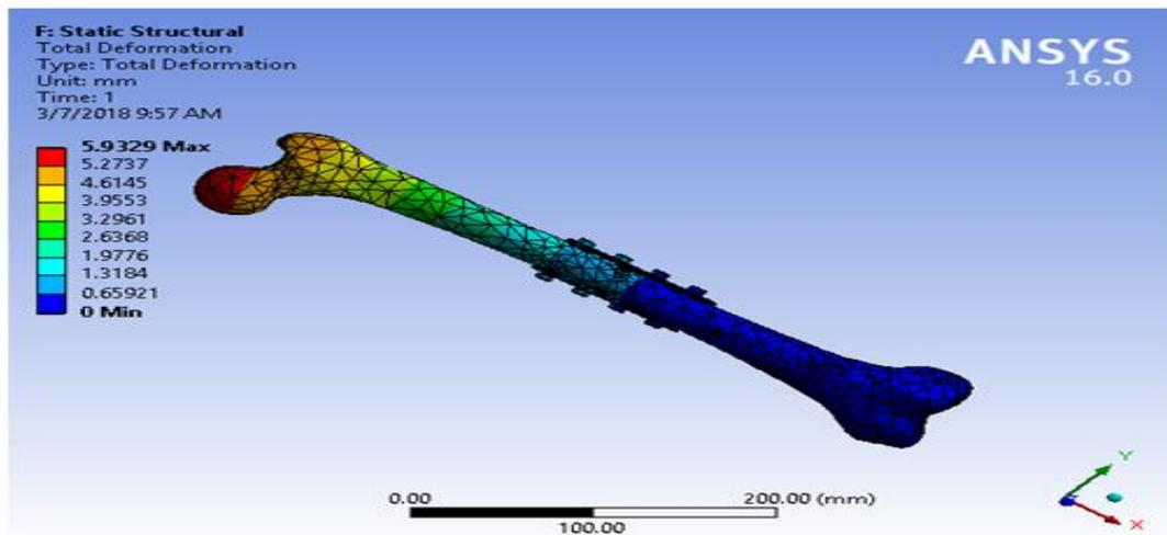
Fig: 4.7.3 picture showing total deformation for model 2 with HP30CF material
