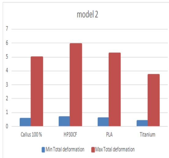
Fig:6 Graph Showing Total deformation For Model 2 with Different Materials
