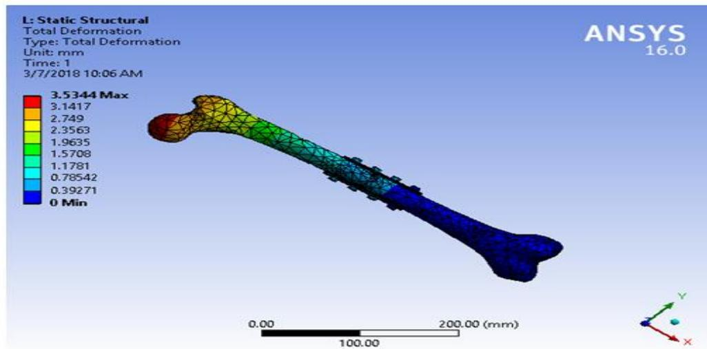
Fig: 4.13.3 Picture showing total deformation for model 3 with titanium materials
