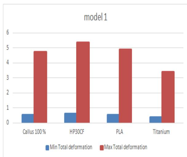
Fig:3 Graph showing Total deformation For Model 1 with Different Materials
