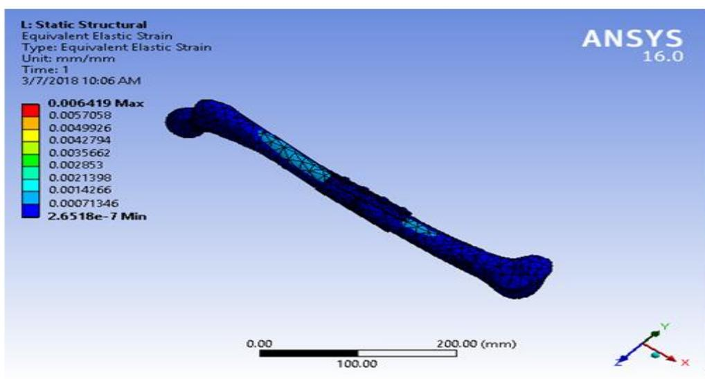
Fig: 4.13.1 picture showing equivalent strain for model 3 with titanium materials
