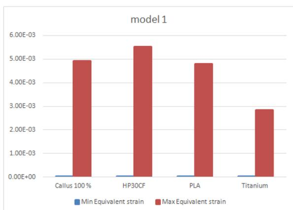
Fig:1 Graph showing Equivalent strain For Model 1 with Different Materials
