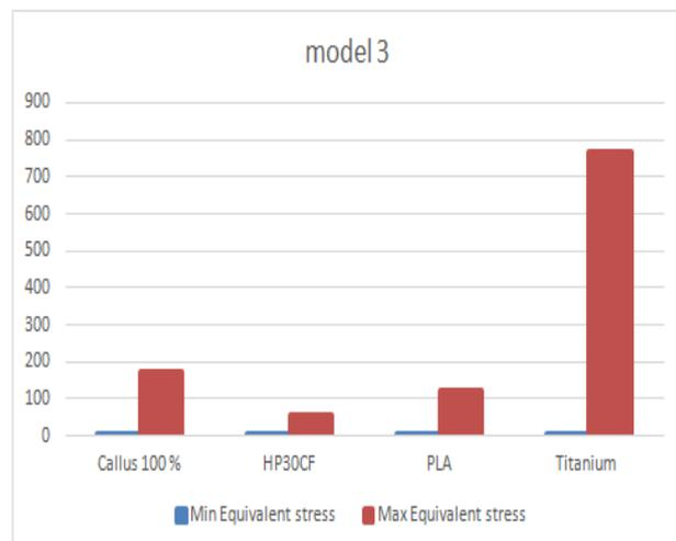
Fig:8 Graph showing Equivalent stress For Model 3 with Different Materials
