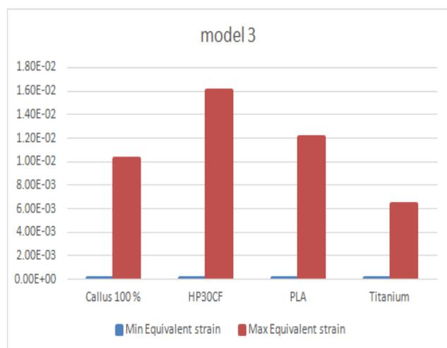
Fig:7 Graph showing Equivalent strain For Model 3 with Different Materials
