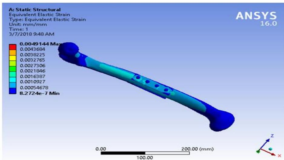
Fig: 4.2.1 picture showing equivalent strain for model 1 with callus(100%)material
