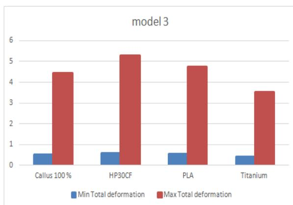
Fig:9 Graph showing Total deformation For Model 3 with Different Material
