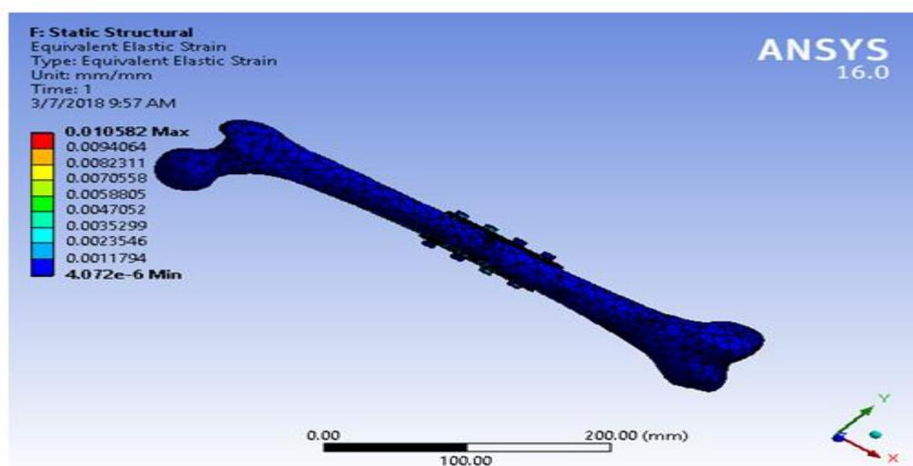
Fig: 4.7.1 picture showing equivalent strain for model 2 with HP30CF material
