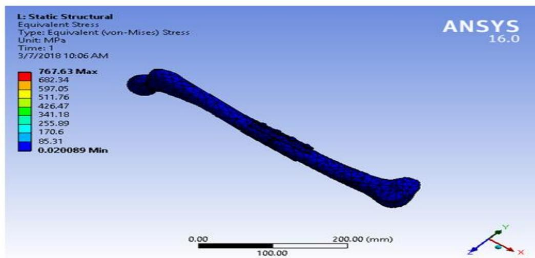
Fig: 4.13.2 graph showing equivalent stress for model 3 with titanium materials
