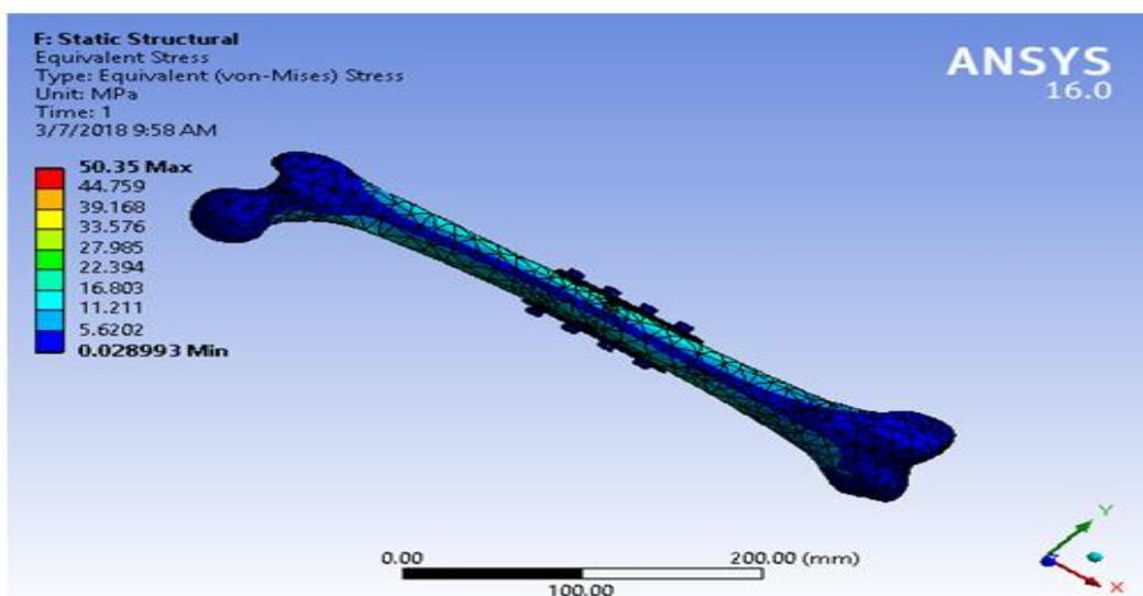
Fig: 4.7.2 picture showing equivalent stress for model 2 with HP30CF material
